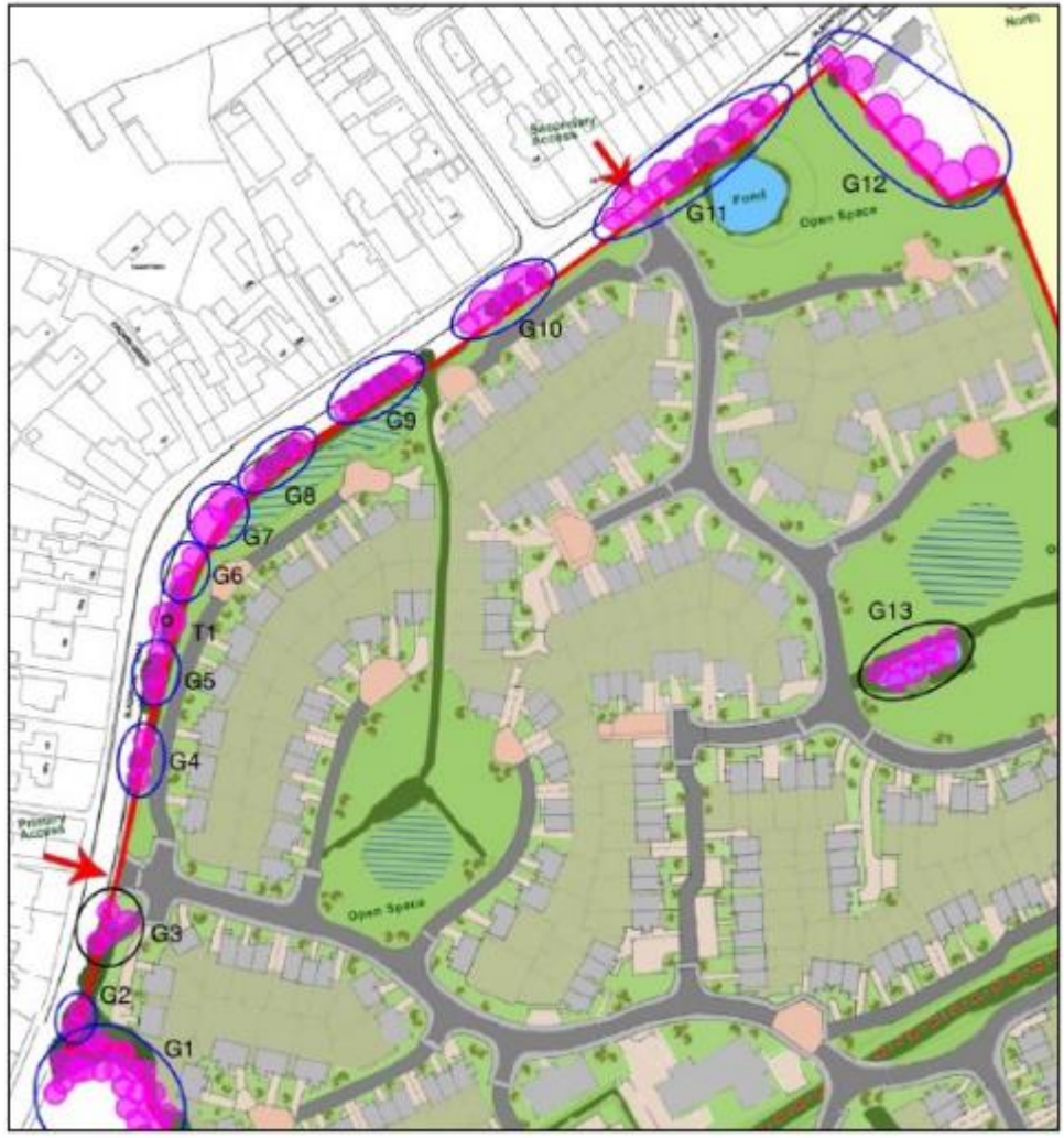
B. An extract from the Tree Report showing the trees surveyed, their groupings and Root Protection Areas (shaded pink) in relation to development proposals
